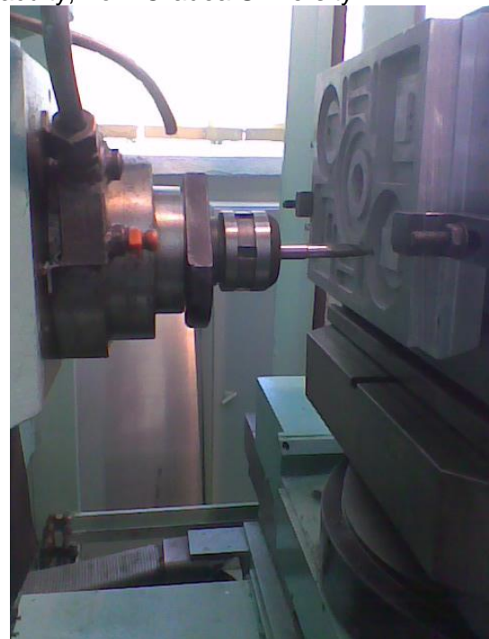
Fig.9. The manufacturing of die on center machine tools.
