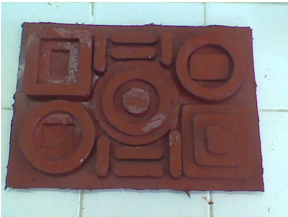
Fig.10. The silicon die for casting of gypsum.
